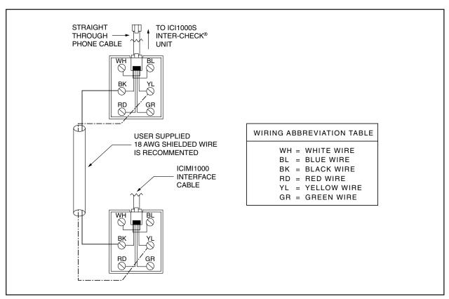
Figure 1. Wiring Diagram for One Cash Register or One ATM Machine
